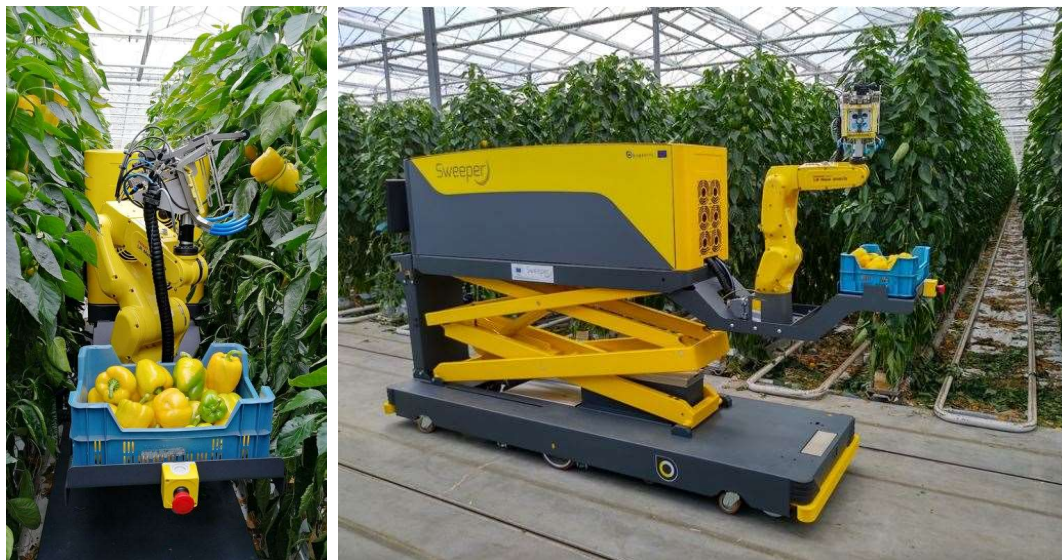
Figure 7 – EU Funded SWEeper Bell Pepper Picking Robot (4,000,000 EUR)
