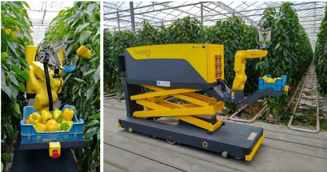
Figure 3 - EU Funded SWEEPER Bell Pepper Picking Robot (4,000,000 EUR)
